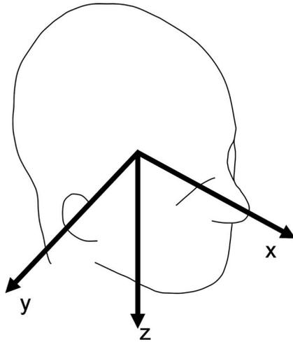
Fig. 2 SAE J211 headform coordinate system
