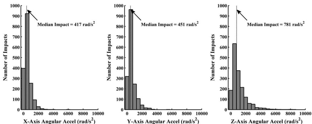
Fig. 5 Distributions of angular acceleration about each axis of the head
