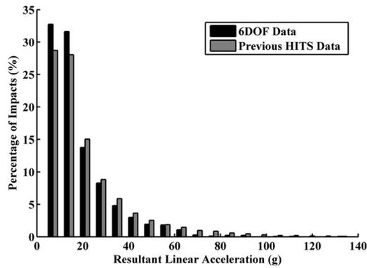
**Fig. 9 Comparison of accelerations collected with the 6DOF measurement device during the 2007 Virginia Tech football season and the original HITS measurement device during the 2003–2006 seasons**
