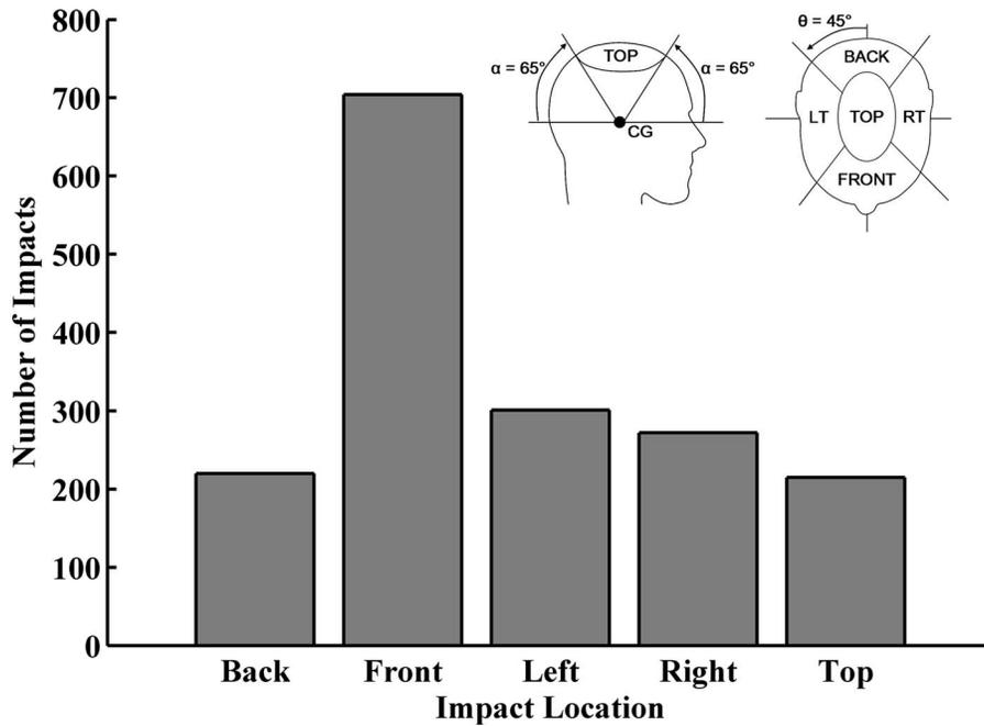
Fig. 6 Distribution of impact locations broken into back, front, left, right, and top bins. Bins are defined in the top right corner of the histogram.
