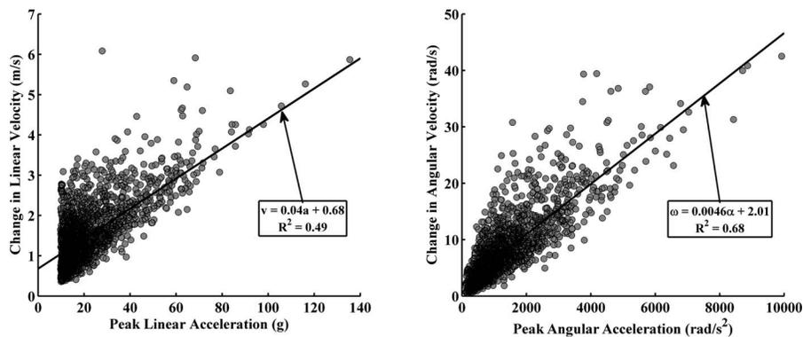
Fig. 8 Relationship between angular change in velocity of the head versus peak linear acceleration (left). Relationship between change in angular velocity of the head and peak angular acceleration (right).
