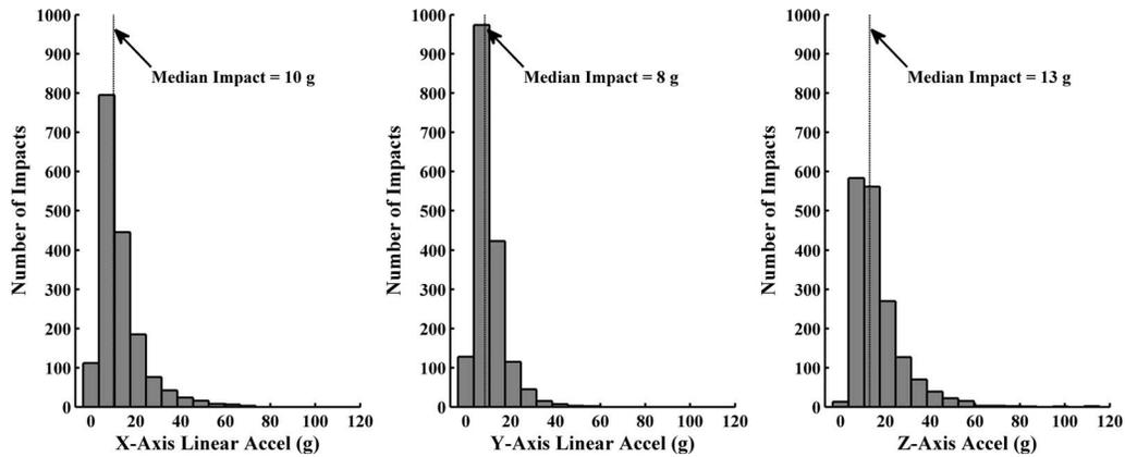
Fig. 4 Distributions of linear accelerations about each axis of the head
