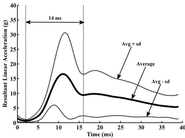
Fig. 7 Average linear acceleration response for the 1712 impacts. The average impact duration was 14 ms.
