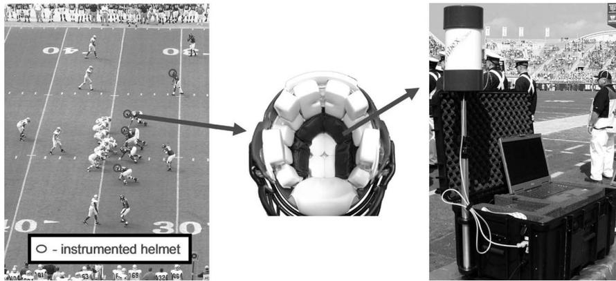
**Fig. 1 Instrumented helmets communicate wirelessly with a computer on the sideline**
