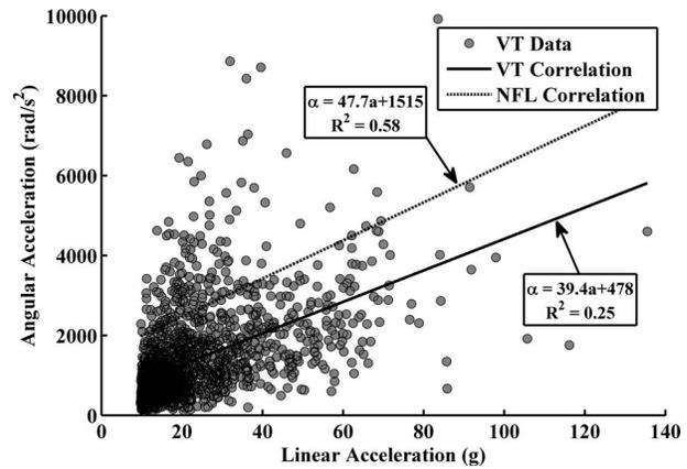
**Fig. 10 Peak angular acceleration as a function of peak linear acceleration. The VT data suggest that no correlation exists ( $R^2=0.25$ ). The dashed line overlays the correlation reported by the NFL study.**
